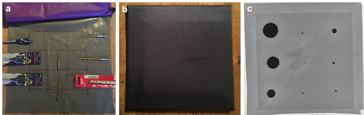
Fig 1. Construction of the detection lead apron phantom for tactile and infrared inspection. (a) Lead apron open exposing 0.5 mm lead-equivalent material (gray) and the backing of the outer apron fabric (purple). A grid is drawn on the material with the drill bit size layout. (b) The shielding material is sandwiched between the apron’s original protective fabric and stapled to a frame. A piece of drywall that is thicker than the frame is placed under the frames cut out to put tension on the fabric and create an “ideal” tactile sensory environment for defect discovery. (c) Radiograph of lead apron phantom.
