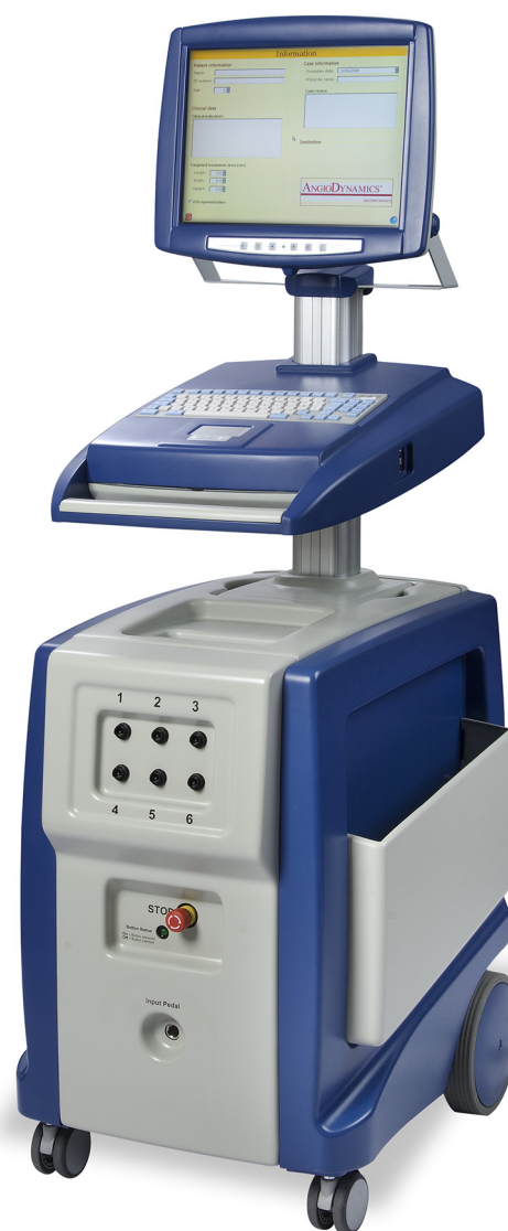
Figure 2 The IRE generator includes an electric power supply, a computer, and 6 output ports that are connected to antennae for the delivery of electric current.
