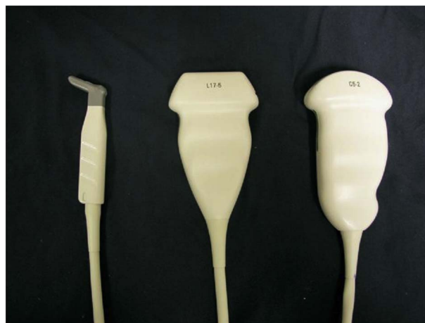
Fig. 1. Commonly used ultrasound transducers in musculoskeletal ultrasound. Left, High-frequency (15-7 MHz), small-footprint, linear array transducer, also called a “hockey stick” transducer. Center, High-frequency (17-5 MHz) linear array transducer. Right, Low-to medium-frequency (5-2 MHz) curvilinear array transducer. Both linear transducers are used for superficial imaging, whereas the curvilinear transducer's lower frequency facilitates examination of deeper regions such as the hip (Philips iU22 Ultrasound Machine; Philips Medical Systems, Bothell, WA).
