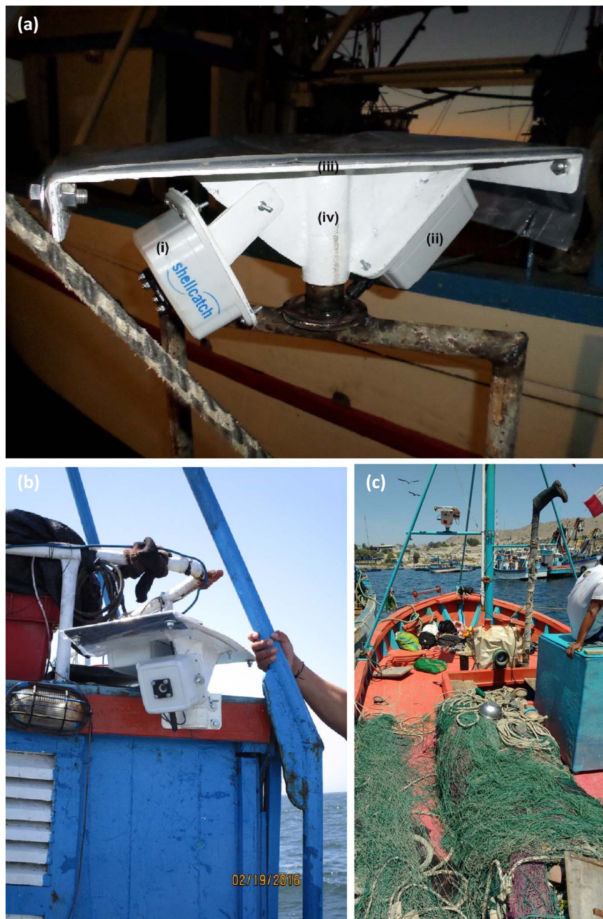
Fig. 1. The camera system developed by Shellcatch Inc. used in our study to monitor catch includes (i) a camera and GPS logger, (ii) a battery pack, (iii) a solar panel to charge the battery, and (iv) a metal frame to mount the camera to the boat. The position where the camera was installed depended on the vessel's configuration. Attachment locations included (a) guard rail (vessel 2); (b) cabin (vessel 3); (c) mast A-frame (vessel 5).
