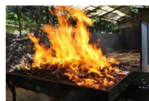
Experimental burning of soil monoliths in a combustion wind tunnel to simulate different fire conditions and different Soil Burn Severity levels
