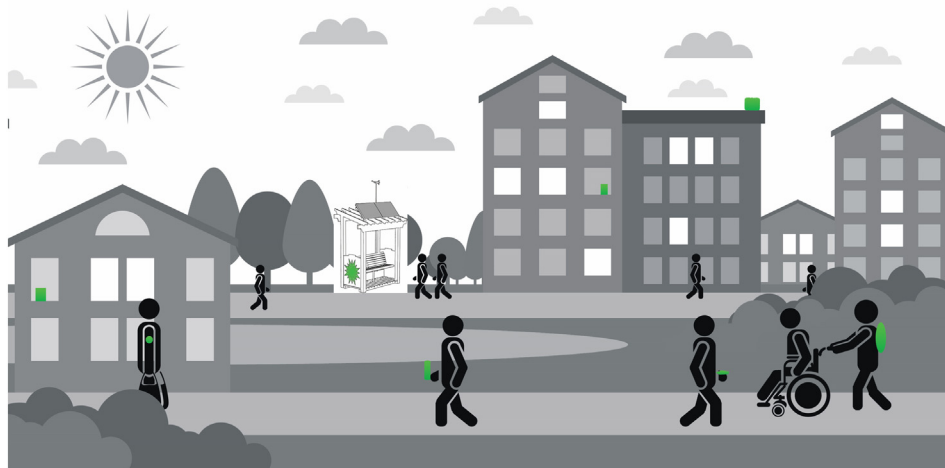
Fig. 1. Low-cost sensors (highlighted in green) provide a wide variety of modes of data collection, including hand-held devices, backpack units, wearable devices, indoor and outdoor fixed devices, and community sensors such as the Village Green sites ( https://www.epa.gov/air-research/village-green-project ). (For interpretation of the references to color in this figure legend, the reader is referred to the web version of this article.)
