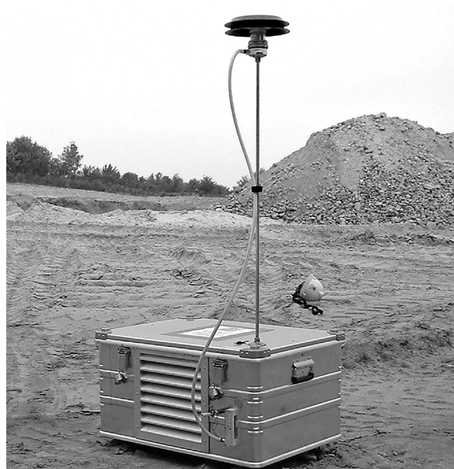
Fig. 1. The HSE high flow rate mobile environmental respirable dust sampler in position at a quarry.
