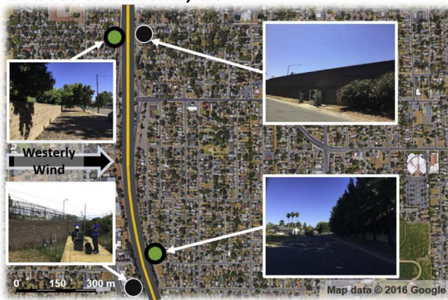
Fig. 1. Aerial images of the study sites near (a) I-101 freeway in Encino and (b) CA-99 freeway in Sacramento. Black and green dots indicate the presence of soundwall and vegetation barriers, respectively. Green dots with black outline indicate the sampling locations with vegetation-soundwall combination barriers. The arrows show the wind directions desirable for the field studies in Encino ( 0 \pm 45^\circ ) and in Sacramento ( 270 \pm 45^\circ ). (For interpretation of the references to color in this figure legend, the reader is referred to the Web version of this article.)
