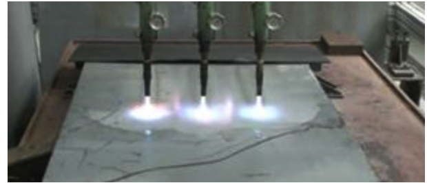
Fig. 3. Scene of multi-line heating test with three torches.
