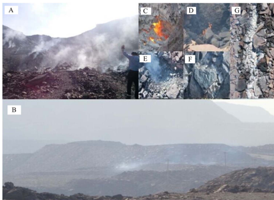
Fig. 1. Landscape and appearance of the coal fire in the Wuda coalfield (A, B: landscape of the Wuda coalfield; C, D: open-flame site; E, F: surface vents with and without smoke, respectively; G: surface cracks).
