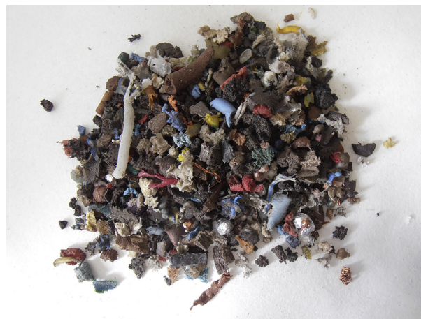
Fig. 1. Polymeric components of cable residue after separation of metals.
