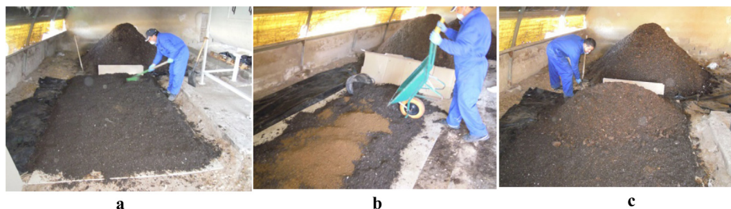
Fig. 1. Image sequence showing the different phases of pilot plant preparation for the production of the biowaste-derived fertilizer. a: preparation of a layer of 40 cm waste mixture at the base of the heap, b: VAP addition in the middle of the heap and c: final heap obtained adding the waste mixture.
