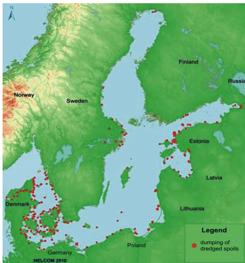
Fig. 1. The storage sites of the dredged sediments in the Baltic Sea according to HELCOM (2010a).
