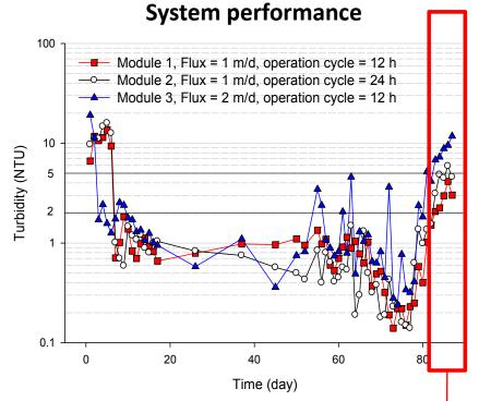
Acceptable start-up duration; High effluent quality during stable operation phase.
