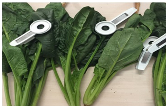
Fig. 1 – Dark-adaptation clips setup in the experiments.
