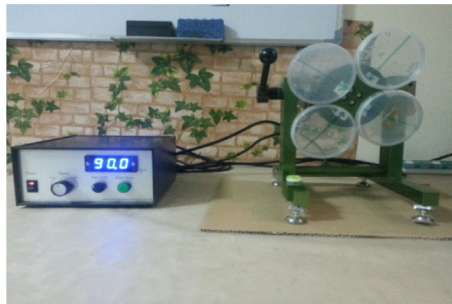
Fig. 1 – Experimental setup of one-axis clinostat.
