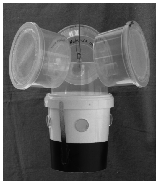
Fig. 1. A multi-chamber trap designed to prevent flies from escaping that remained active for a long time after feeding on bait without knockdown properties placed in the removable black base.
