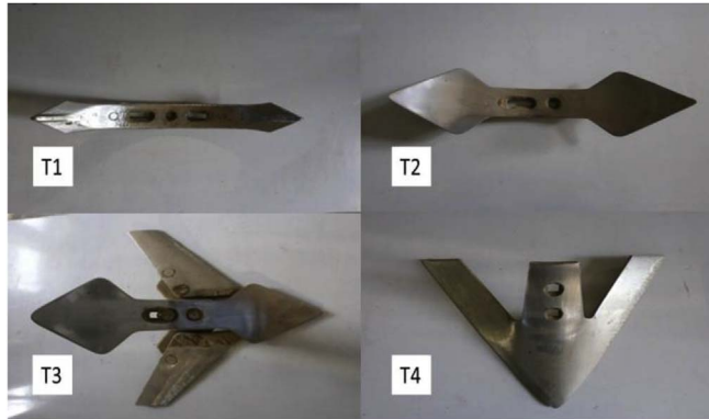
Fig. 1. Tines used T1) heavy duty, T2) double heart, T3) double heart with wings and T4) duck foot.
