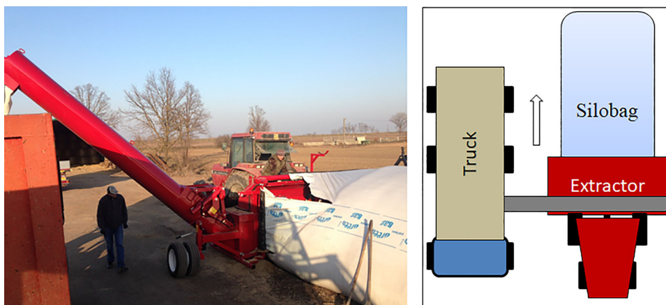
Fig. 1. View of the extractor during the unloading (left) and scheme of the configuration at work (right).
