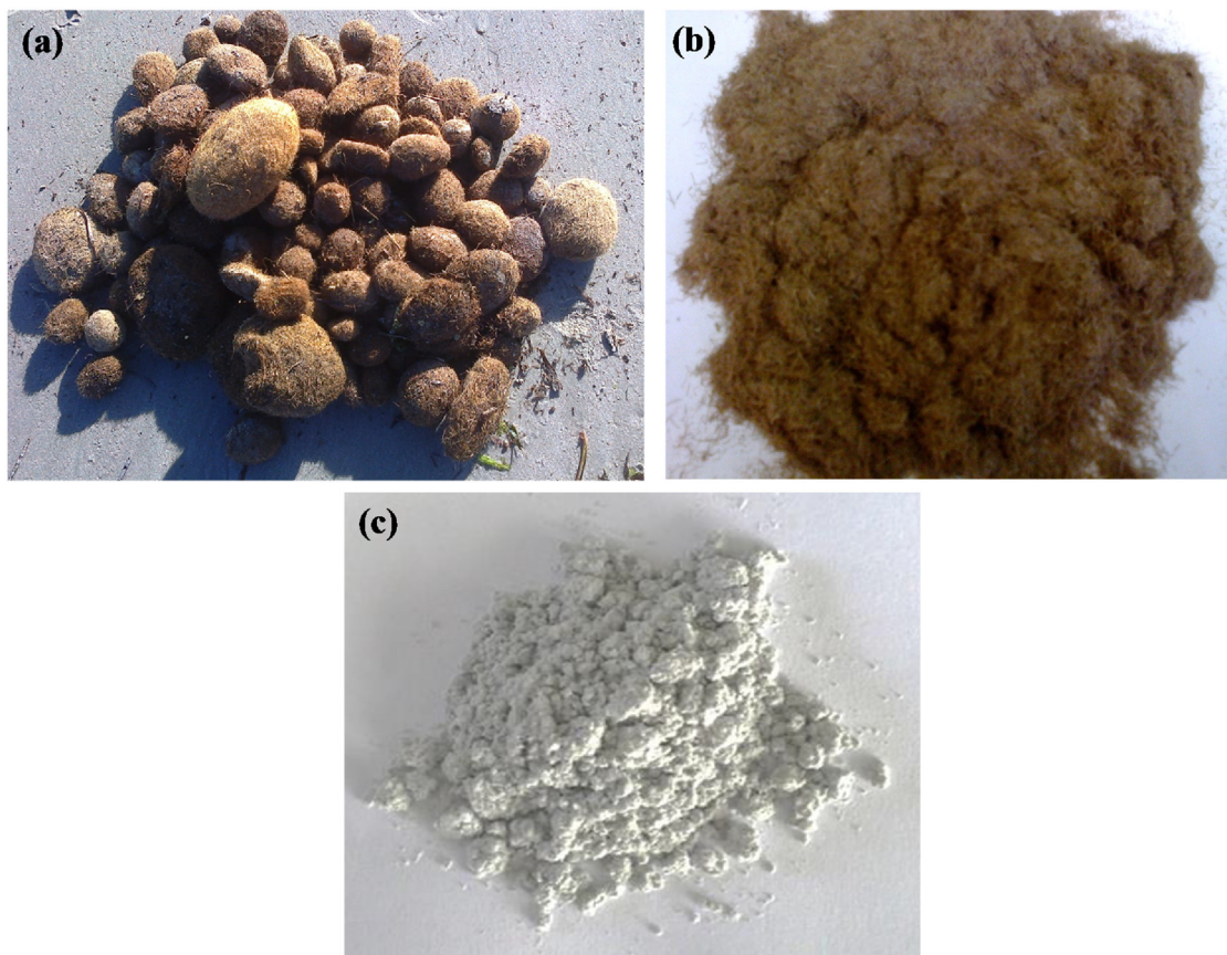
Fig. 1. Filler images ((a) Posidonia oceanica balls, (b) Posidonia oceanica fibres (POF) and (c) Raw DPS).
