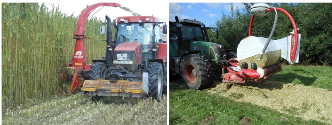
Fig. 1. Harvest of hemp with a field chopper (left) and densification as well as wet preservation of the chopped harvest material (right).
