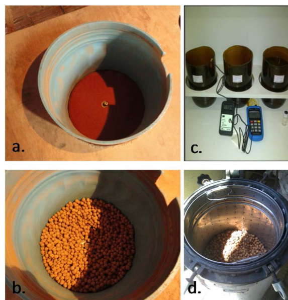
Fig. 1. Mechanical extraction process: (a) Circular bench sander and (b) Fiber extraction; Chemical mercerization process (NaOH autoclave): (c) 0.5% NaOH solution and (d) autoclave.
