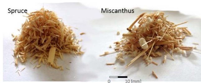
Fig. 1. Spruce and Miscanthus particles as used for particleboards.
