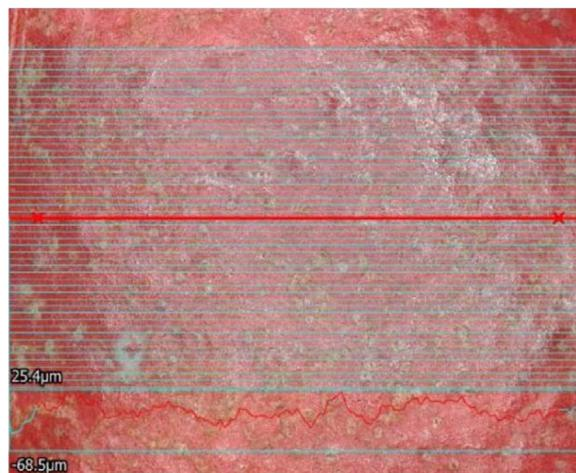
Fig. 2. Split beam technology of the 3D profilometer showing the 51 lines on the pomegranate peel to determine the fruit surface roughness.
