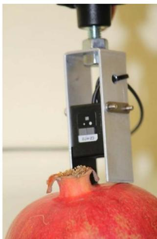
Fig. 1. Gloss measurement using the luster sensor technology and a) measuring scheme, b) the newly machined distance holder.
