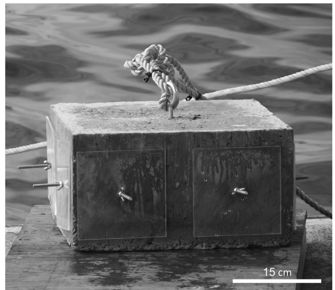
Fig. 1. Fouling panel and cement block design. Rope is attached to a surface float (outside picture). Photo by J. Reynolds.
