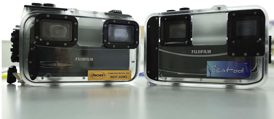
Fig. 1. Fujifilm FinePix Real 3D W1 (right) and W3 (left) stereo cameras housed in waterproof cases.
