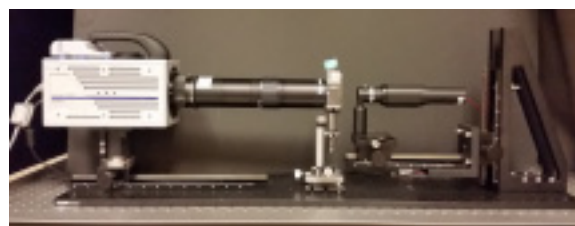
Fig. 1. The high-speed microscale imaging system (HSMIS).
