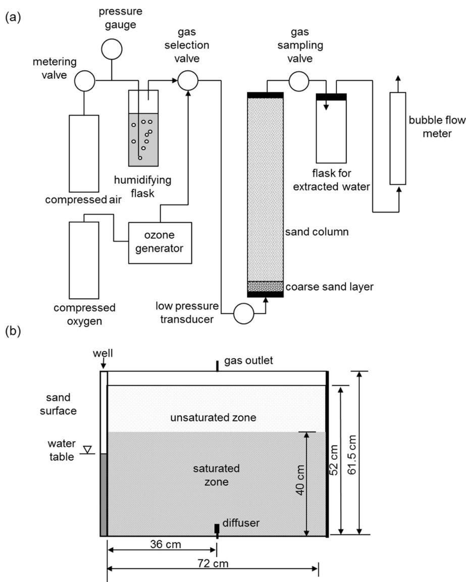
Fig. 1. Schematic diagram of experimental set up: (a) air sparging system with 1-D column installed, (b) dimensions of 2-D model with the heights of sand packing, saturated zone, and the water table.
