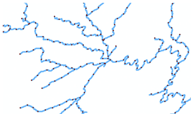
Fig. 1. Illustration of the stream-network splitting procedure. Points are generated on top of the stream network line features at user-defined distances (e.g. 50 km), the point layer is used to split each feature.
