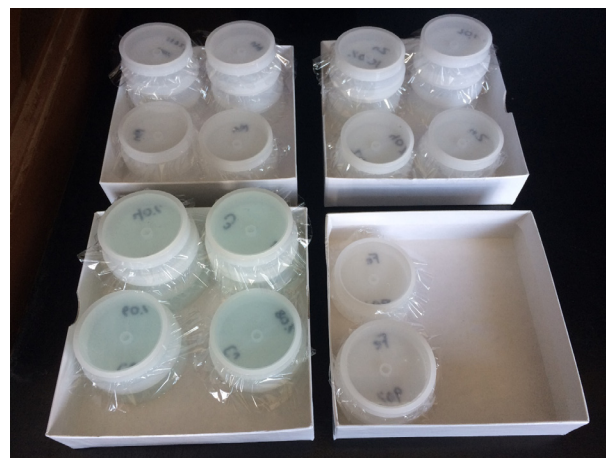
Fig. 1. Water samples placed in Series 1400 plastic sample cups and covered with Prolene® thin-film.
