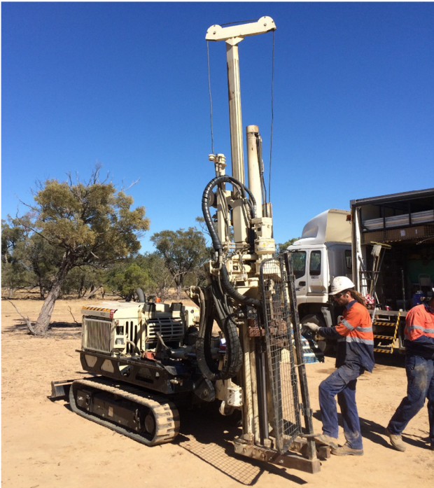
Fig. 1. Direct push drilling of the alluvial aquifer on the floodplain of the Flinders River using a Geoprobe Systems 7822DT rig.
