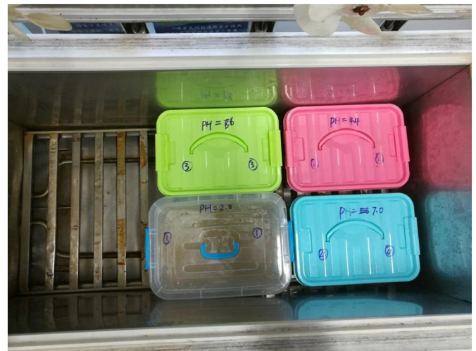
Fig. 2. The samples in the freeze-thaw test machine.
