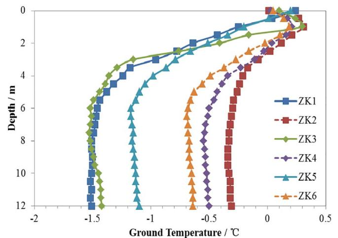
Fig. 2. Ground temperature profiles of the typical boreholes in permafrost regions.
