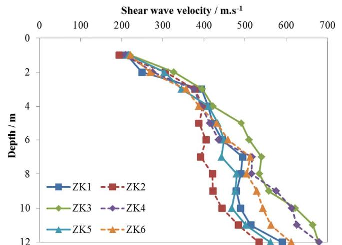
Fig. 1. The variations of shear wave velocity with depth of the typical boreholes.
