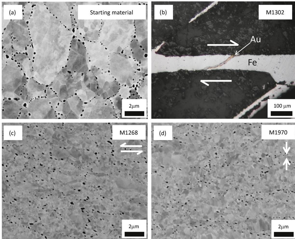
**Fig. 1.** (a) Back-scattered electron image (BEI) of the starting material, namely Fe. (b) Optical microscopic image and (c) BEI of samples recovered from shear deformation experiments of Fe (b, M1302; c, M1268). (d) BEI of the sample recovered from the uniaxial deformation experiment of Fe (M1970).
