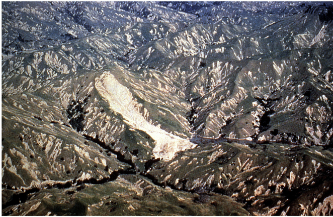
Fig. 1. A large, multiple-occurrence regional landslide event resulting from Cyclone Bola rainfall of 300–900 mm in 72 h, affecting an area of over 8300 km 2 , March 1988, East Coast, North Island, New Zealand (photo: Noel Trustrum).
