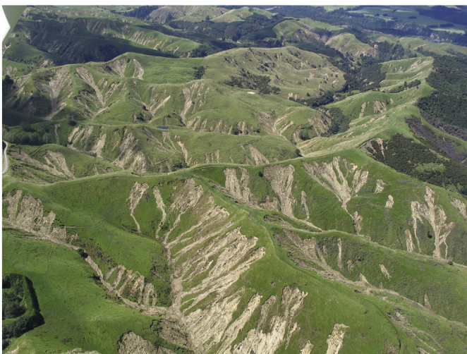
Fig. 2. Landslides resulting from the Wanganui-Manawatu event of February 2004; rainfall exceeded 300 mm in 72 h in the worst affected areas. Landslide locations are aligned to drainage lines and to ridge crests (photo: Graham Hancox).
