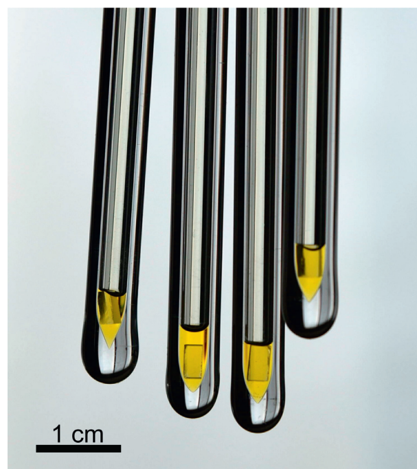
Fig. 1. Quartz glass pressure vessels for pure Cl_2 experiments. A rectangular WP obsidian slab is immersed in liquid Cl_2 . The space above the liquid is filled with Cl_2 gas. A similar experimental setup was used for other experimental series.
