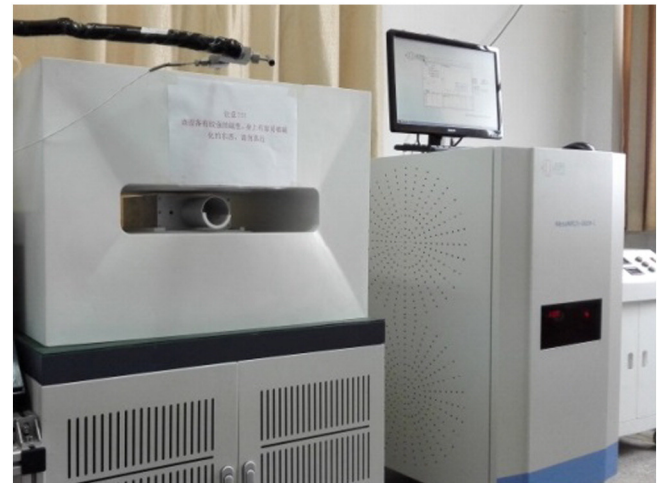
Fig. 3. Nuclear magnetic resonance (NMR) instrument.
