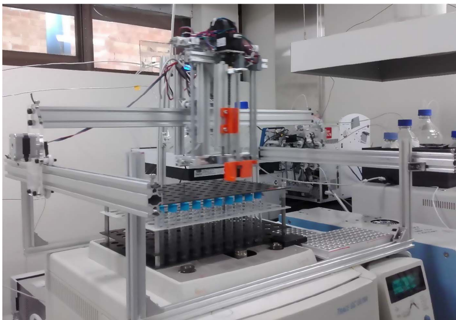
Fig. 1. Osmar, the open-source microsyringe autosampler mounted on top of a gas chromatograph.
