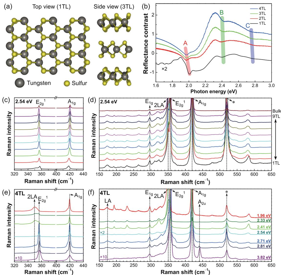
**Fig. 1.** (a) Crystal structure of monolayer (top view) and 3TL (side view) WS<sub>2</sub>. (b) Reflectance contrast spectra of 1TL to 4TL. Thickness dependence of Raman spectrum of (c) main peaks ( $E_{2g}^{-1}$  and  $A_{1g}$ ) and (d) weaker peaks measured with 2.54 eV excitation. Excitation energy dependence of Raman spectrum of 4TL WS<sub>2</sub> for (e) main peaks and (f) weaker peaks. The silicon signal at 520 cm<sup>-1</sup> is marked by \*.
