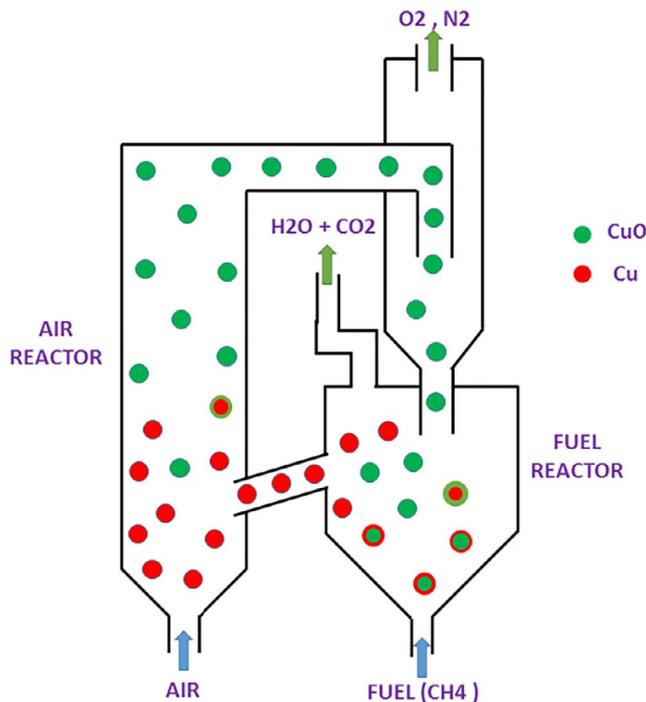
Fig. 1. Fluidized bed reactors in a CLC system.
