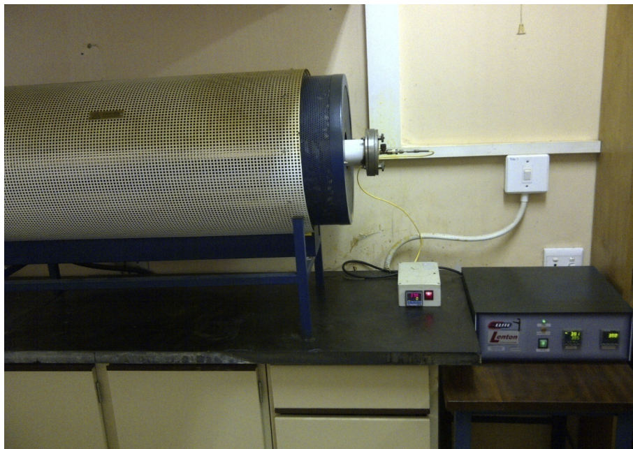
Fig. 1. Tube furnace used for char preparation.
