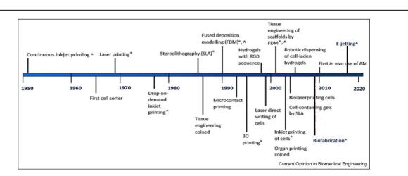
Evolution of additive printing technologies. \* used for bone tissue engineering, ^ used for tendon tissue engineering (Figure is adapted with permission from [6]).
