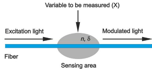
Fig. 3. Idea of operation optical fiber intrinsic sensor.
