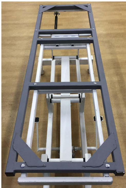
Fig. 2. Original two-section treatment plinth base-frame (white) and one fabricated steel frame (grey).
