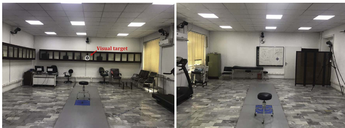
Fig. 1. Musculoskeletal biomechanics laboratory in which the measurement procedures were performed. Six cameras were set up and angled in a manner to decrease hidden spots that might obscure data collection. In addition, a visual target (white A4 paper with a black circle drawn upon it) was used to standardize head posture.
