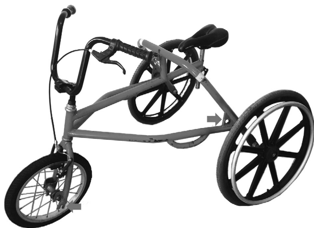
Figure 1 Illustration of the non-pedal tricycle adapted for the study. Note: The arrows indicate the adaptation made to enable adjustments to the front and back wheels in order to have the non-pedal tricycle either higher or lower depending on the height of the user.
