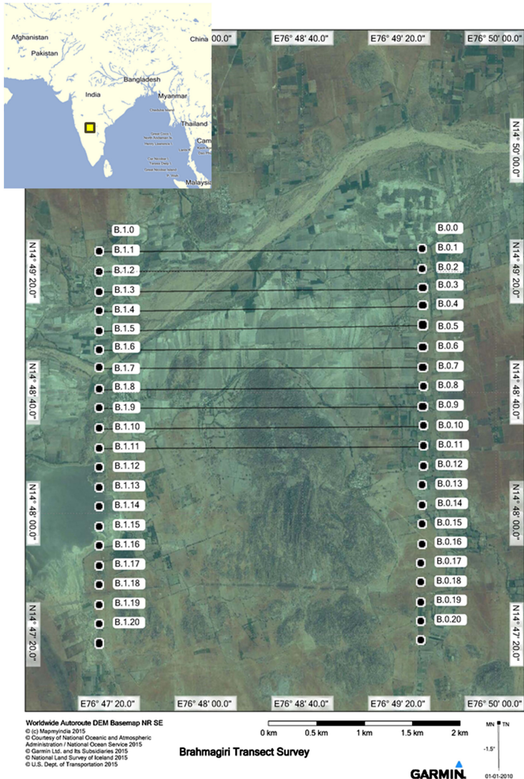
Fig. 1. Transect survey area of 16 km 2 (4 × 4 km), centring Brahmagiri hill and covering riverbanks of Hagari, plains and clusters of small granitic hillocks. The transect lines each are 4 km in stretch spaced at 200 m intervals. The drawn transect lines indicate area so far covered.
