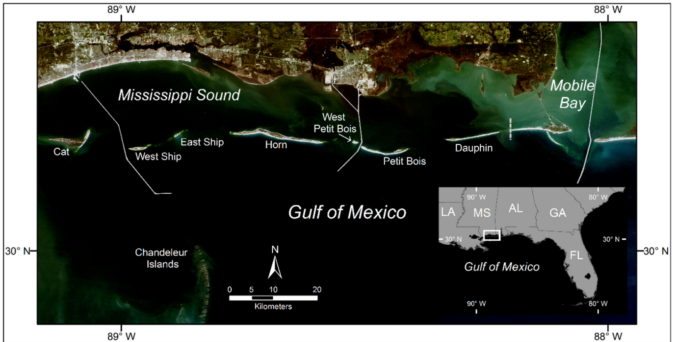
Fig. 1. Landsat 5 Thematic Mapper (TM5) natural color image of the MS-AL barrier islands and mainland coast acquired on 16th September 2005, approximately two weeks after the 29th August 2005 Mississippi landfall of Hurricane Katrina. By acting as sediment traps, ship navigation channels (solid white lines) extending from Mobile Bay and west of Petit Bois and W. Ship islands have increasingly reduced the volume of westward-directed net longshore sediment transport since the late 19th century (Morton, 2008). Erosional conversion of most of the Chantelaur Islands, Louisiana to sandy shoals (Otvos and Carter, 2013; Moore et al., 2014; Otvos, 2018a, in press) rendered them barely visible at bottom-left in the image. The dashed vertical white line on Dauphin Island indicates longitude 88.2° W, the eastern limit of the study area.
