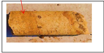
Sandstone core extracted from 32.5 m depth (area # 3, borehole # 8)
