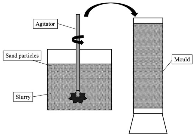
Fig. 1. Schematic diagram of the mixing process.
